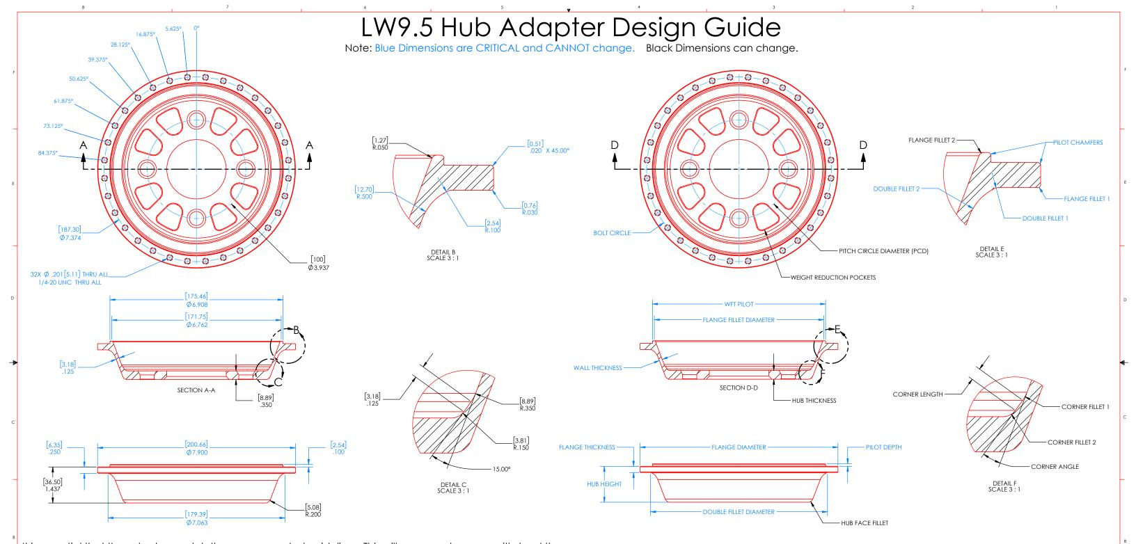
It is essential that the adapters match the recommended guidelines. This will ensure system can withstand the rated loads and provide the most accurate results. The critical features are shown in blue. Customers may change all other geometry. Examples of permitted changes are shown on the second sheet,
